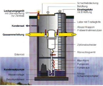
Figure 4– Condensate shaft
