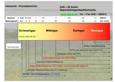
Figure 9 – Operation range of gas utilisation facilities
