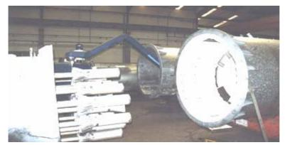
Figure 8 – Ceramic lining inside the flare stack (insulation liner)
