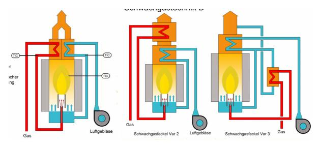
Figure 11 – Different heat exchanger systems for low calorific flares
